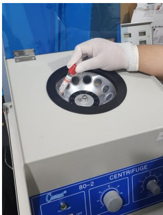
Figure 3. Blood is centrifuged using a Corona® centrifuge at a speed of 3000 rpm for 10 minutes to obtain the serum.
