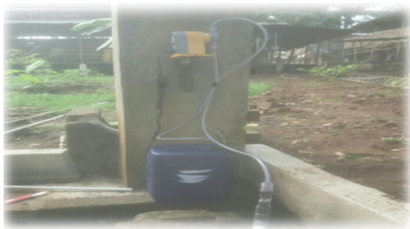
Figure 1. Dosing equipment using hydrogen peroxide disinfectant
