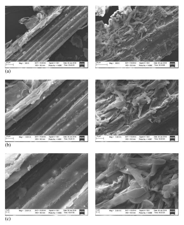
Figure 2. Scanning electron microscopy (SEM) of untreated oil palm frond (left) and treated oil palm frond with FCT + 5% urea (right) at 500× (a), 1,000× (b) and 2,000× (c) magnification.
