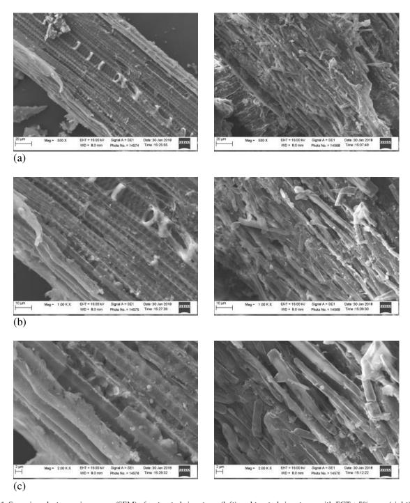
Figure 1. Scanning electron microscopy (SEM) of untreated rice straw (left) and treated rice straw with FCT + 5% urea (right) at  $500 \times (a)$ ,  $1,000 \times (b)$  and  $2,000 \times (c)$  magnification.
