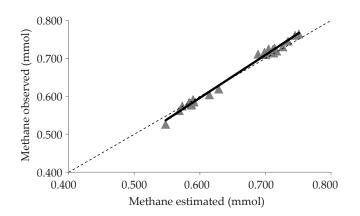
Figure 2. Plot between estimated (from volatile fatty acid profile) and observed (using infrared methane analyzer) methane emission. Regression equation: Methane observed= -0.084 + 1.133 × Methane estimated (P<0.001; R<sup>2</sup>= 0.992; RMSPE= 1.75%). Dashed line indicates an ideal line where the estimated methane emission is equal to the observed methane emission.
