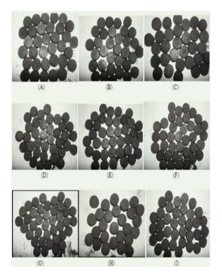
Figure 2. Biopelet of palm shell with the formulation palm shell: palm shell charcoal: palm fiber (A) 100:0:0 (B) 90:0:10; (C) 80:0:20; (D) 90:10:0; (E) 80:10:10 (F) 70:10:20; (G) 80:20:0; (H) 70:20:10; (I) 60:20:20
