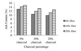
Figure 4. The effect of the percentage of palm shell, palm shell charcoal, and palm fibers to the ash content of biopellet
