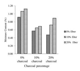
Figure 3. The effect of the percentage of palm shell, palm shell charcoal, and palm fibers to the moisture content of biopellet
