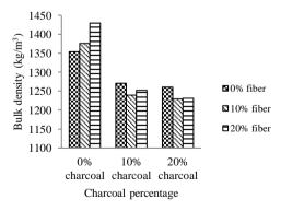
Figure 8. The effect of the percentage of palm shell, palm shell charcoal, and palm fibers to the bulk density of biopellet
