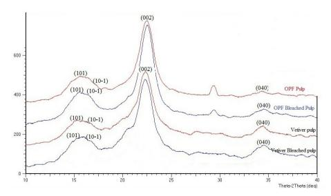
Figure 3. X ray diffractogram of soda pulp and bleached soda pulp from OPF and dVR
