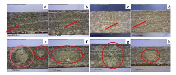
Figure 8. Micrograph of cross sectional surface before mechanical testing of (a) PP/OPF-unbleached-fibrillatedpulp, (b) PP/OPF-unbleached-pressed-pulp, (c) PP/OPF-bleached-fibrillated-pulp, (d) PP/OPFbleached-pressed-pulp, (e) PP/dVR-unbleached-fibrillated-pulp, (f) PP/dVR-unbleached-pressed-pulp, (g) PP/dVR-bleached-fibrillated-pulp, (h) PP/dVR-bleached-pressed-pulp composites
