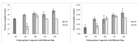
Figure 4. (a) Flexural strength and (b) flexural modulus of composite from PP with filler from pulp of OPF or dVR in form of fibrillated-unbleached (FU), fibrillated-bleached (FB), pressed-unbleached (PU), pressed-bleached (PB)
