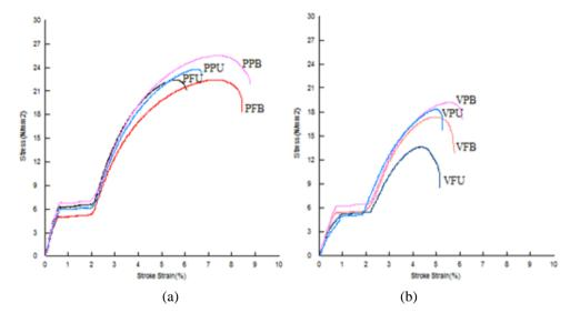
Figure 7. Stress-Strain graph of tensile properties of (a) PP/OPF composites (b) PP/dVR composites
