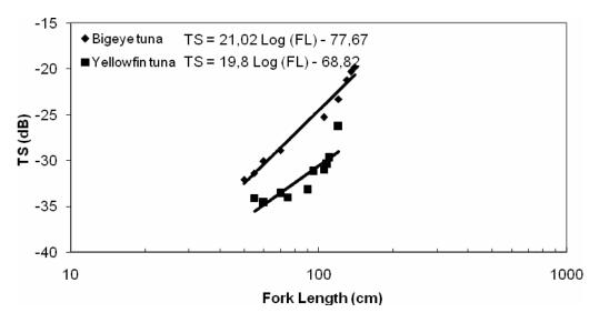
Figure 2. Variation of target strength with tuna fork length (cm) for bigeye and yellowfin tuna. Solid line is the best fit equation  $TS = a \log FL + b$  of experimental data. x-axis is a logarithmic scale.
