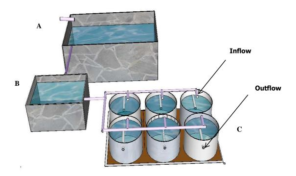
Figure 1. The integrated tank-based aquaculture system for the marine fish and seaweed culture experiments. A. fish tank, B. sediment tank, C. seaweed tanks.
