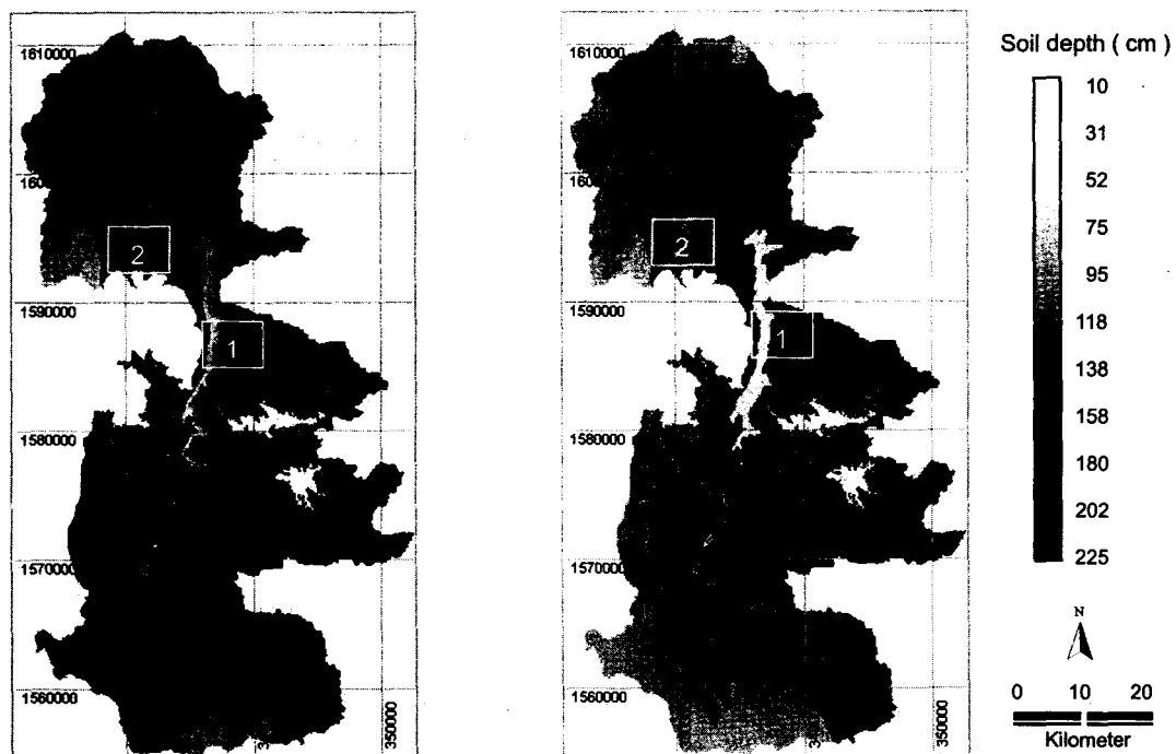
Figure 4. Soil depth of the study area derived from membership maps (left) and conventional map (right). Boxes indicate the sample areas for complex topography (box 1) and flat lowland (box 2)
