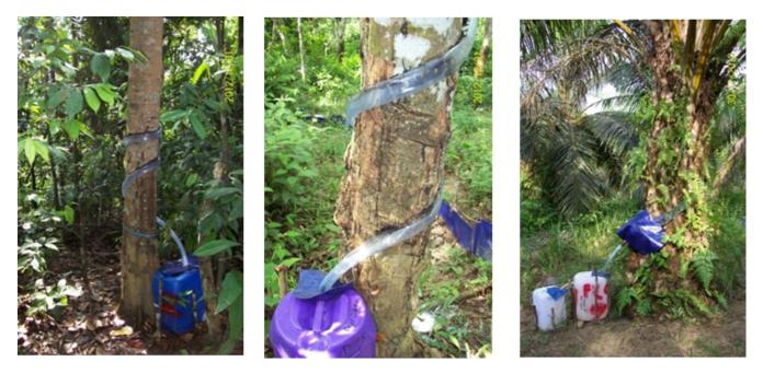
Figure 1 Setting up the measurement tool of stemflow volume.
