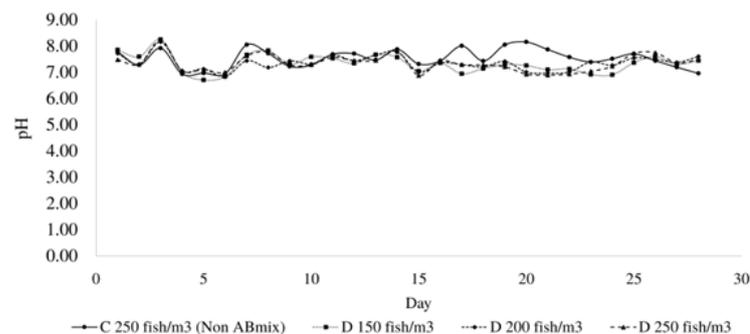
Figure 1. The pH value of *Clarias* sp. rearing water at various levels of stocking density with the aquaponics system for 28 days.
