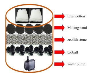
Figure 2. Filtering drum composition.
