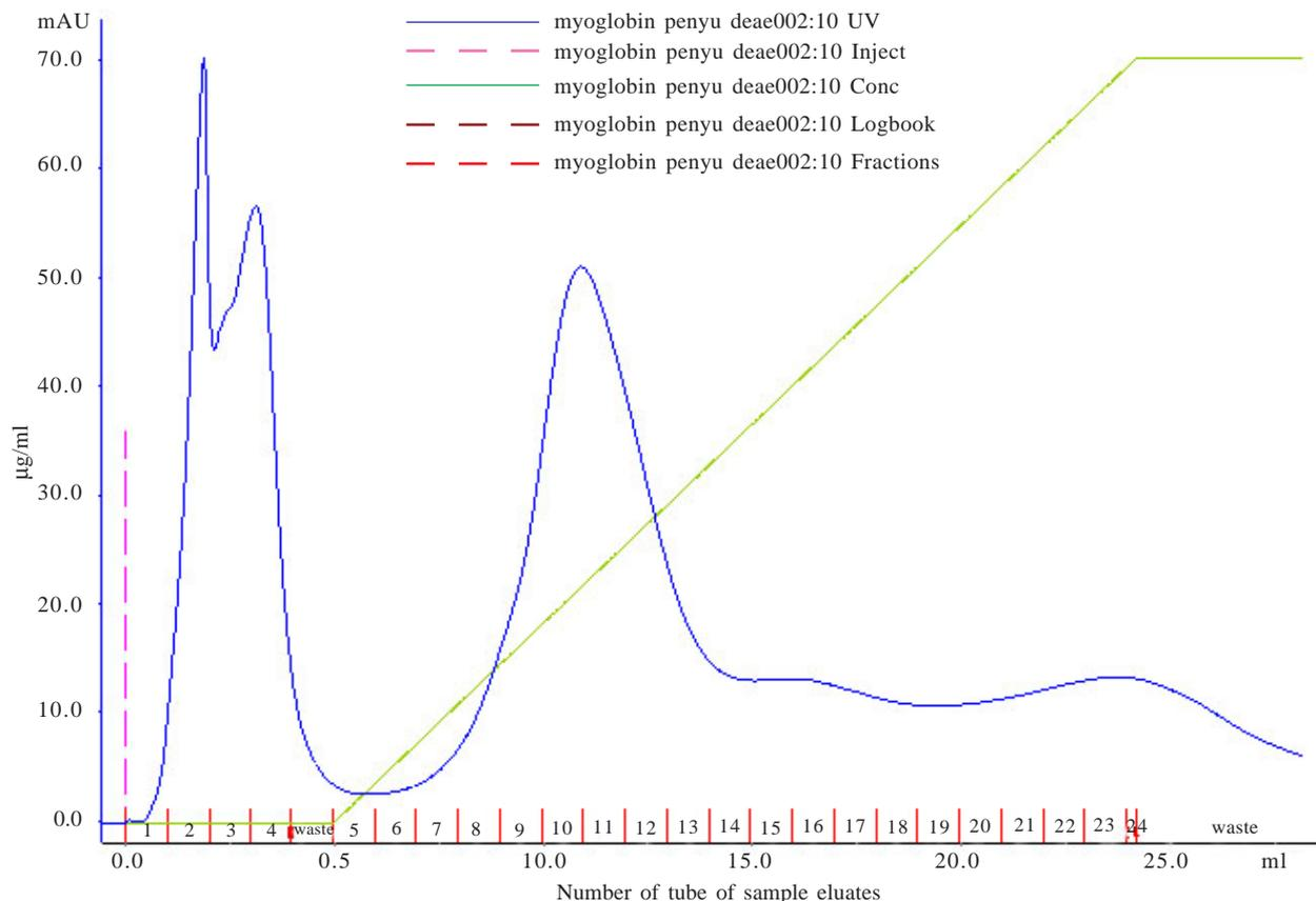
Figure 4. Separation of Mb with DEAE-Sephrose by using AKTA Purifier-Amersham.
