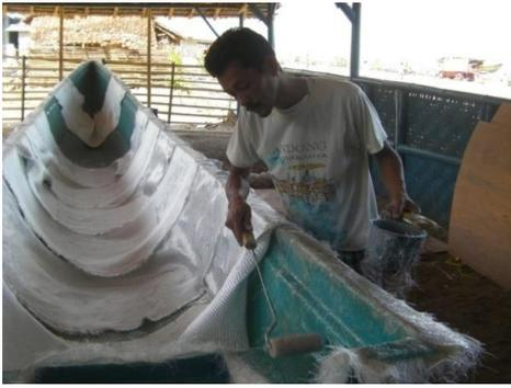
Gambar 5 Pelapisan *mat* dan *roving*
